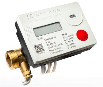
The LYKH series ultrasonic thermal energy meter uses state-of-the-art technology to ensure the accurate measurement of energy usage. The meter has no moving parts, and it uses an innovative time differential measuring principle. With dual register capabilities, the meter can record both heating and cooling consumption in hydronic systems with a seasonal changeover, as well as in traditional 4-pipe systems.
